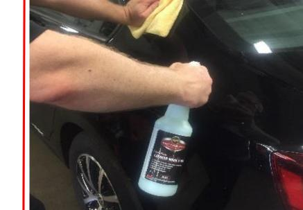
Shake well: For use with rotary with Polishing Foam pad WRFP7 & Backing Plate WRSBP Work one section at a time. Apply product onto a cool surface. Work in 2x2 foot areas. Work area until nearly dry. Wipe off excess with a clean Supreme Shine Microfiber X2020, Maximum 1600 rpm. Or use the MT300 with DMC5/6 pad at 4800 OPM's following same procedure.
