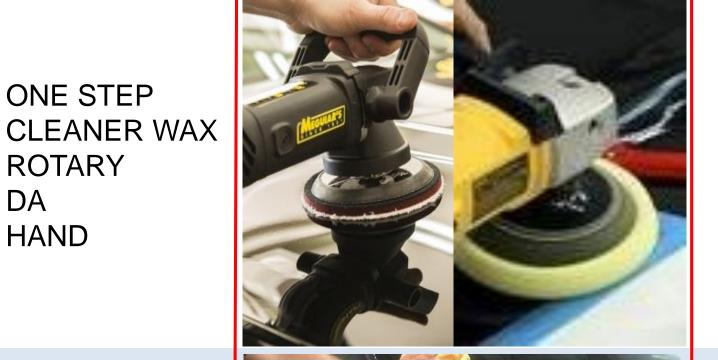
Apply M21 Synthetic Sealant with DA polisher set on 3800 OPM using a DFF5 Foam Finishing Pad (black). Apply product to entire vehicle then wipe off with X2020 Supreme Shine Microfiber Towel.
